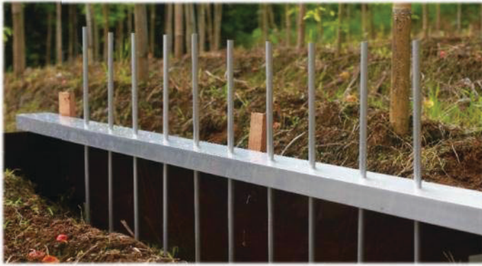
Figure 4. The modified erosion bar used in monitoring soil erosion. (Adapted from Ramirez, 1988 as cited by Visco, 1997)
