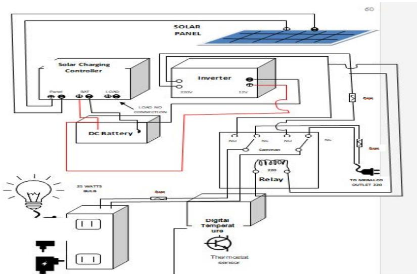
Figure 3. Circuit Diagram of Microgrid in a Small Poultry with Temperature
