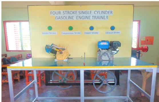
Figure 2. This four Stroke single Cylinder gasoline Engine - Section Model displays internal combustion (IC) engine in which the piston completes four separate strokes while turning the crankshaft; simulations work as it is powered by the functional engine.
