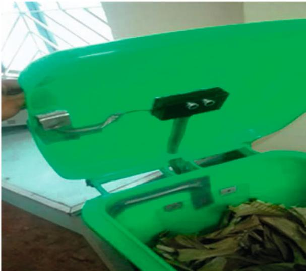
Figure 9. Smart Bin with ultrasonic sensor equipped at surface level
