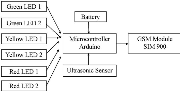
Figure 8. System Block Diagram
