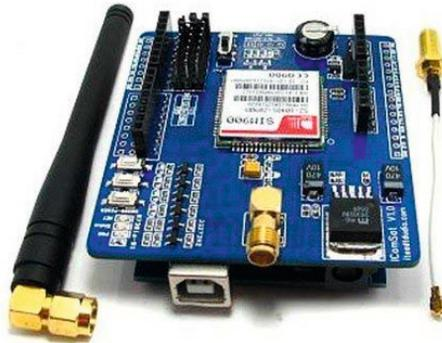
Figure 2. GSM Module SIM900
