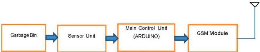
Figure 5. Transmitter Block Diagram
