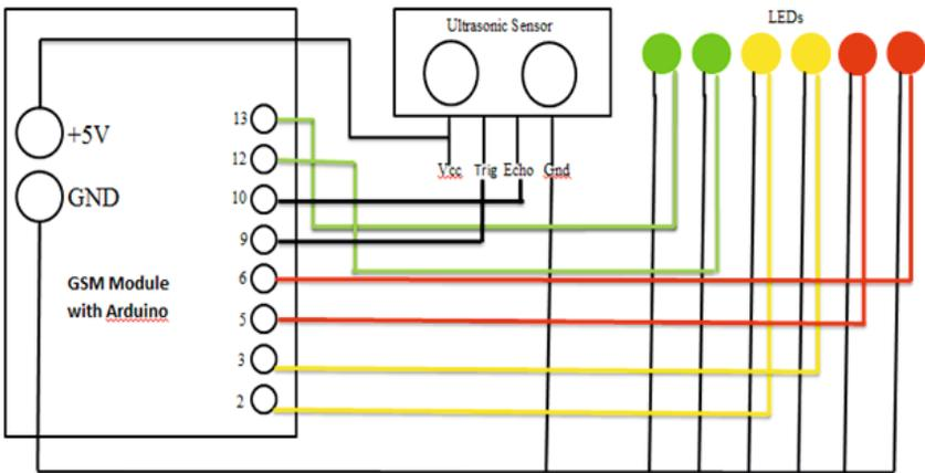
Figure 7. GSM Module with Arduino Ultrasonic Hardware Connection
