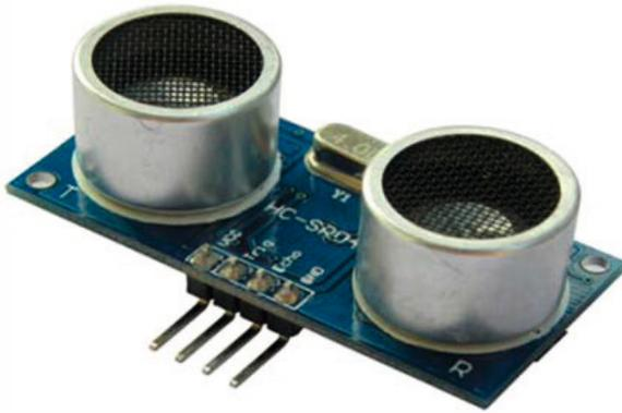
Figure 4. Ultrasonic Ranging Module HC - SR04
