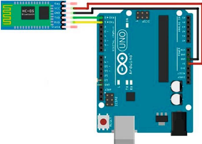
Figure 9. Arduino Bluetooth hardware Connection
