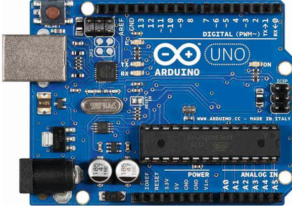
Figure 4. Arduino microcontroller
