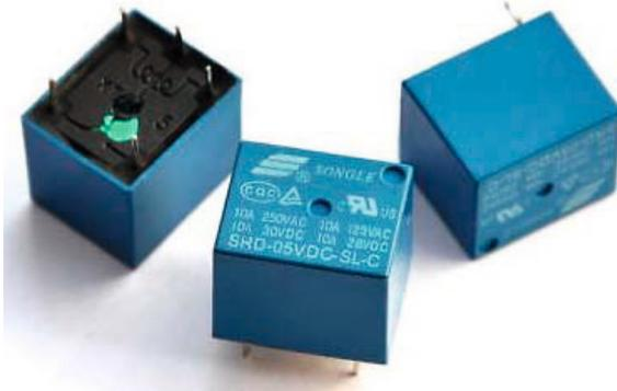
Figure 11. Single-pole double-throw (SPDT) 5V Relays
