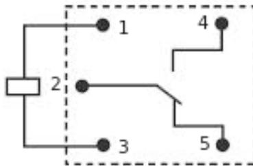
Figure 12. Relay pin-out
