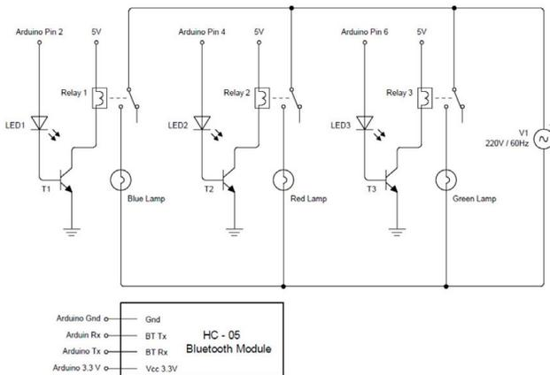
Figure 10. Lighting System Schematic Diagram
