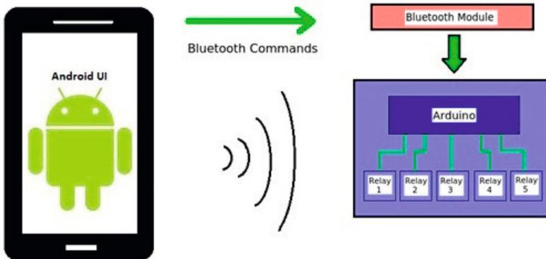
Figure 8. Automatic Lighting System Block diagram
