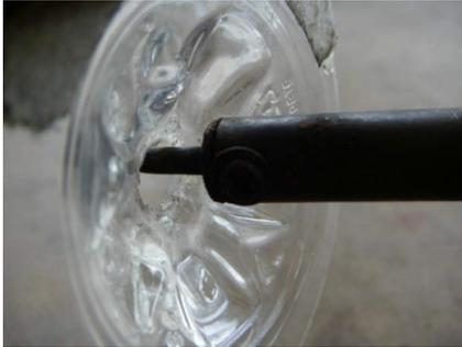
Figure 22. Cutting the Center Spot using a soldering iron
