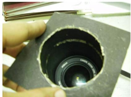
Figure 12. Mount the filter holder to the Camera
