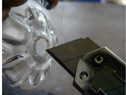
Figure 23. Cutting the Center Spot using a hand cutter to make the hole smoother
