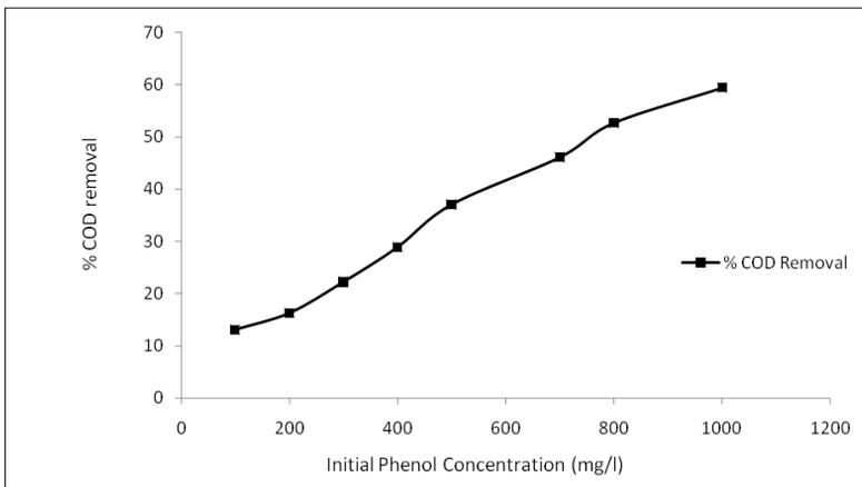
Figure 1. COD Percentage Removal during Adaptation of Phenolic Wastewater
