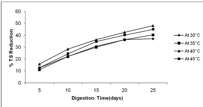
Figure 4. Effect of digestion time on percentage TS Reduction at four different temperatures
