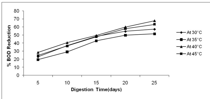
Figure 2. Effect of digestion time on percentage BOD Reduction at four different temperatures
