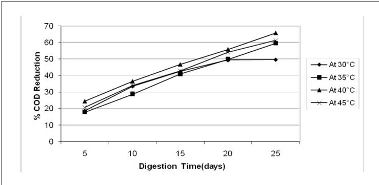
Figure 3. Effect of digestion time on percentage COD Reduction at four different temperatures
