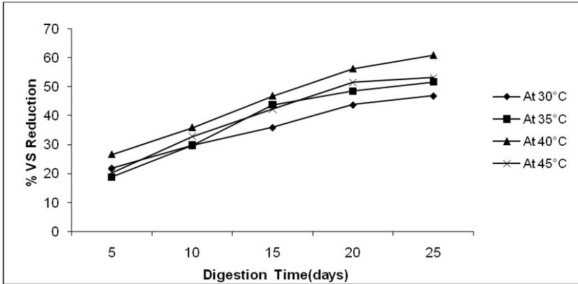
Figure 6. Effect of digestion time on percentage VS Reduction at four different temperatures
