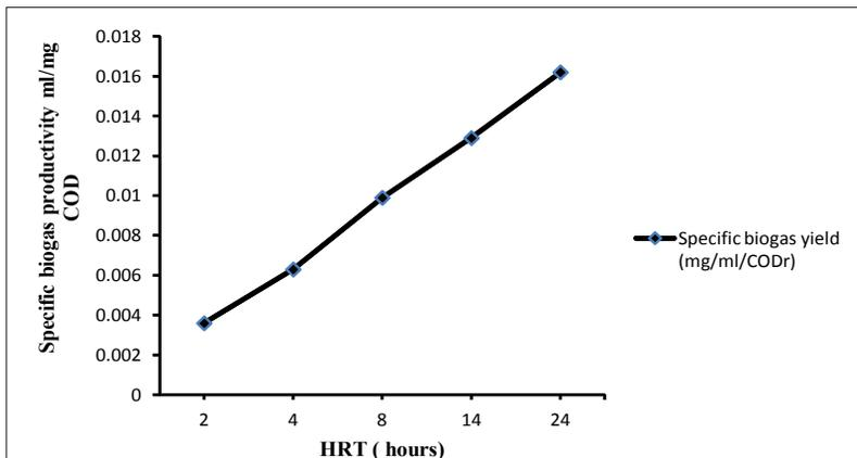
Figure 9. Effect of hydraulic retention time on specific biogas productivity
