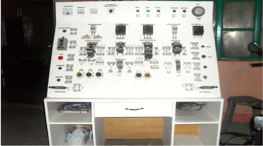
Figure 2. Electric motor controller trainer an instructional device
