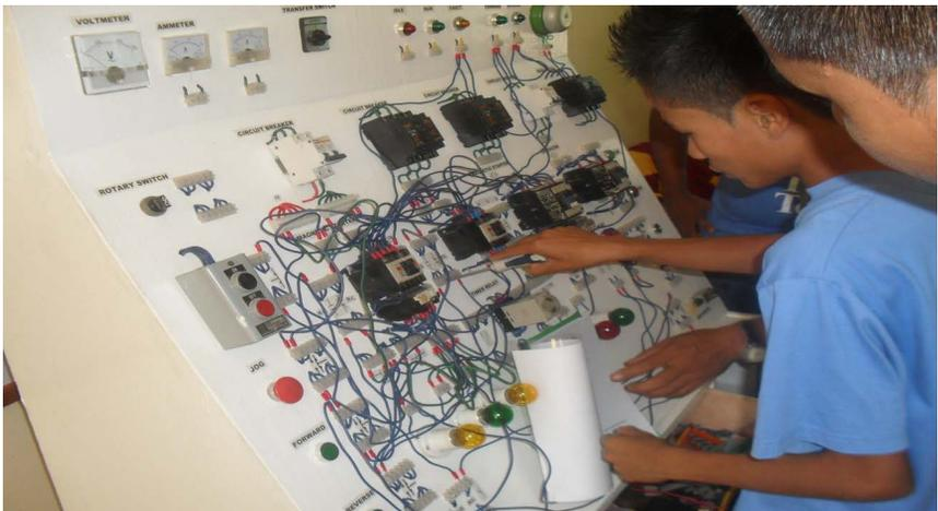
Figure 3. Student is performing “START-STOP, Full-Voltage Starter with Alarm Silencing” at the newly constructed trainer
