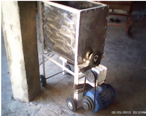
Figure 3. Installation of gear box and motor
